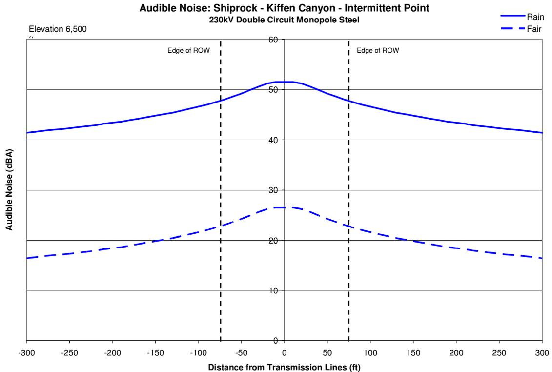
The results of the corona audible noise modeling plotted in Figure 9 show that on both ROW edges the audible noise is approximately 23 dBA in fair weather and 48 dBA in wet weather.
