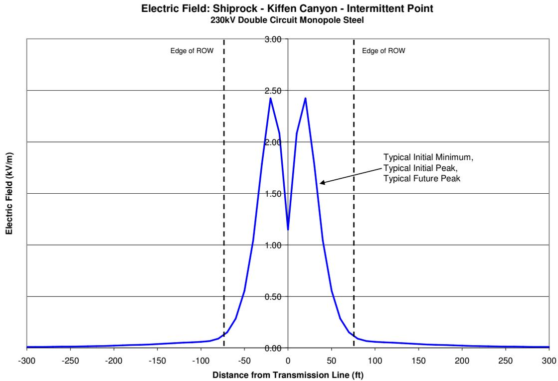
The results of the electric field modeling plotted in Figure 1 show that on both ROW edges the electric field is approximately 0.1 kilovolt per meter (kV/m) for all three power flow cases. This is because electric fields do not vary with power flow. The maximum electric field within the ROW is 2.4 kV/m.
