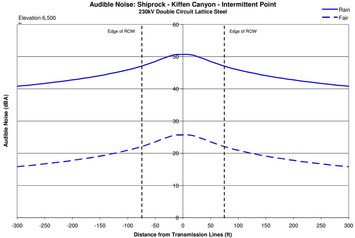
The results of the corona audible noise modeling plotted in Figure 10 show that on both ROW edges the audible noise is approximately 22 dBA in fair weather and 47 dBA in wet weather. The maximum noise that occurs within the ROW is 25.7 dBA in fair weather and 50.7 dBA in wet weather.
