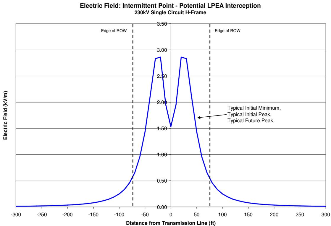
The results of the electric field modeling plotted in Figure 5 show that on both ROW edges the electric field is approximately 0.55 kV/m for all three power flow cases. This is because electric fields do not vary with power flow. The maximum electric field within the ROW is 2.9 kV/m.
