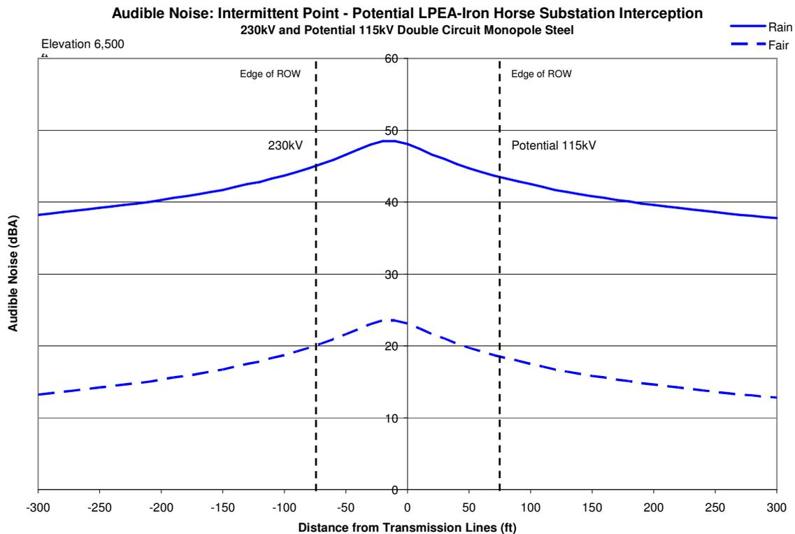
The results of the corona audible noise modeling plotted in Figure 12 show that on the left ROW edge the audible noise is approximately 20 dBA in fair weather and 45 dBA in wet weather. Figure 12 shows that on the right ROW edge the audible noise is approximately 19 dBA in fair weather and 43 dBA in wet weather. The curves are shifted slightly to the left because the 230 kV circuit on the left side will produce slightly more corona noise than will
