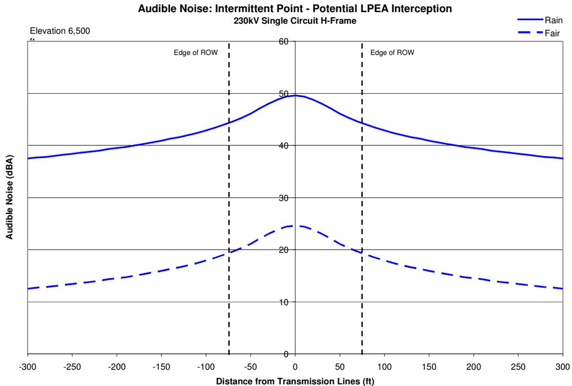
The results of the corona audible noise modeling plotted in Figure 11 show that on both ROW edges the audible noise is approximately 19 dBA in fair weather and 44 dBA in wet weather. The maximum noise that occurs within the ROW is 24.6 dBA in fair weather and 49.6 dBA in wet weather.
