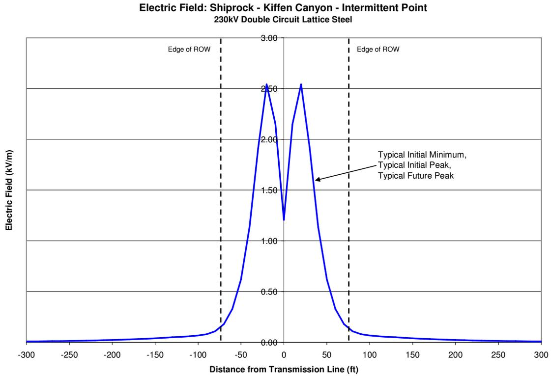
The results of the electric field modeling plotted in Figure 3 show that on both ROW edges the electric field is approximately 0.15 kV/m for all three power flow cases. This is because electric fields do not vary with power flow. The maximum electric field within the ROW is 2.5 kV/m.
