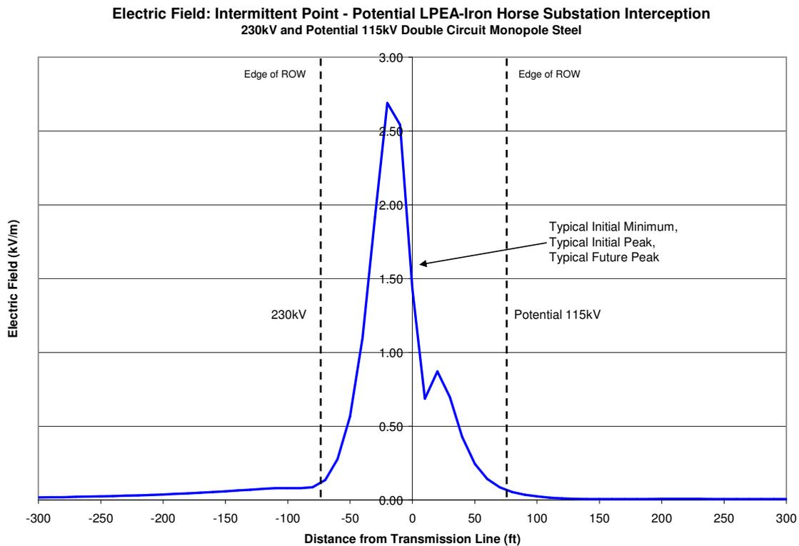
The results of the electric field modeling plotted in Figure 7 show that on the left ROW edge the electric field is approximately 0.11 kV/m for all three power flow cases. Figure 7 shows that on the right ROW edge the electric field is approximately 0.07 kV/m for all three power flow cases. The reason for this shift is that the 230 kV circuit on the left side of the structures will produce a higher electric field than will the 115 kV circuit on the right. Electric fields do
